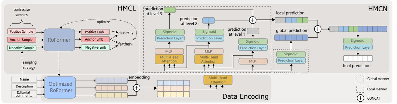
**Figure 3: The HMCL + HMCN architecture. In HMCN, the left dotted block refers to the local manner, and the right dotted block refers to global one. The Prediction Layer refers to the last MLP layer for prediction, and  $\oplus$  indicates a CONCAT operation.**
