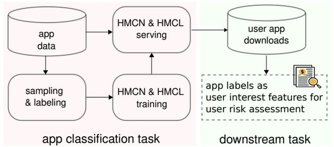
**Figure 4: The deployment of the HMCN and HMCL, and the role of its app classifications in the downstream task of user risk assessment. The app labels assigned by the HMCN are used to extract user interests from the app download history of users, which are then merged with additional features for training and inference of the risk assessment model.**
